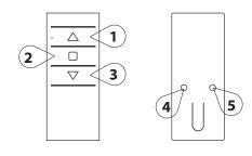
The buttons shown on the left are used to program the transmitters and specific channels. The programing button's (buttons 4 and 5) locations can be placed differently depending on the transmitter model. Shown in this guide is the Emitto Slim line transmitter.
