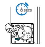
Repeat steps 1-6 for all motors. Once complete Press and hold the Lock button for 6 seconds while looking at the LED, and hold until solid.
