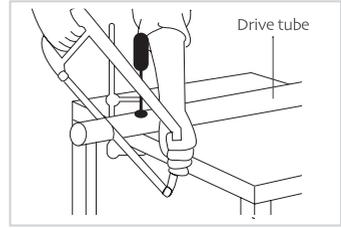
**Step 2.** Ensure roller tube is clean and free from burrs.
