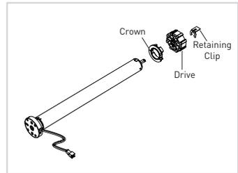
**Step 4.** Slide Motor into tube.
