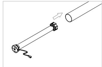
**Step 5.** Mount motorized tube onto brackets.
