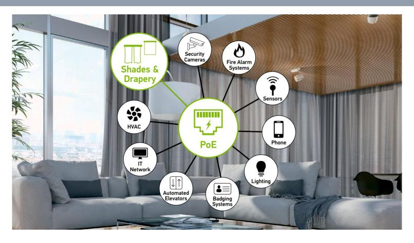
Power over Ethernet (PoE) distributes network signals and electrical power to transmit communication over standard low-voltage category cabling to various endpoints, including shades, draperies, LED lighting, HVAC controls, cameras and other networked devices in new or existing projects.
