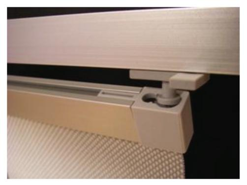
First push the pin on the slider in to the bigger hole of the panel holder plug. After that push the panel towards the slider. There should be a snap, when the pin of the slider clicks in to the panel holder plug correctly. The folded ends of the fabric should be on the reverse side of the completed product.
